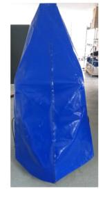
To make it easier to put on the cover, it is equipped with a zip fastener on the side of the machine arm.
