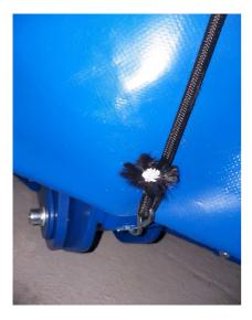
The cover is attached to the minicrane by means of 5 elastic tensioners: 4 attached to the suport feet and one to the wheel.
